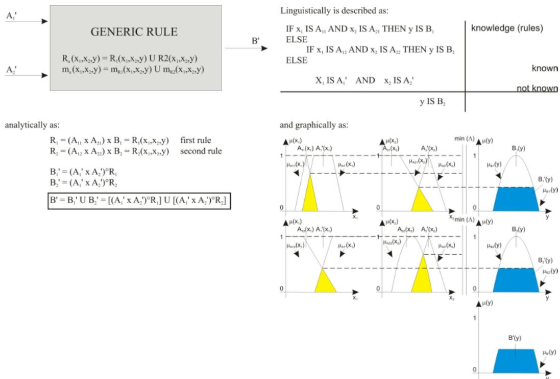
Figure10: GMP with many inputs and many rules
