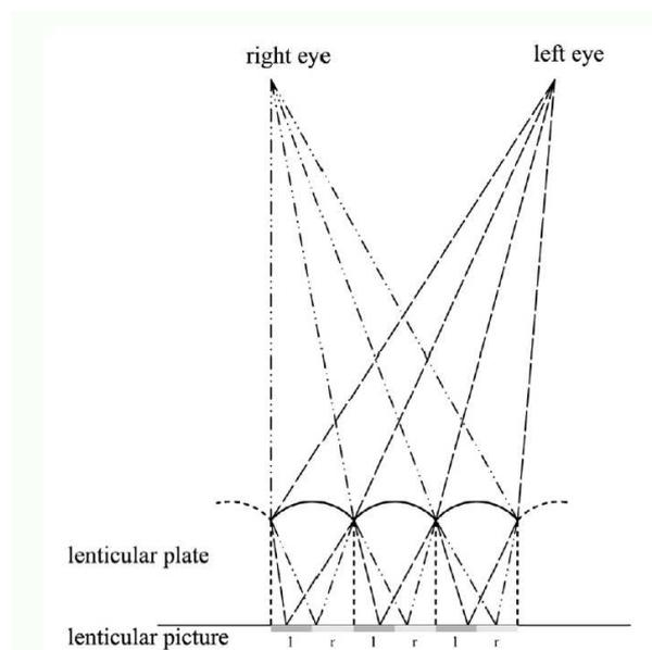
Fig. 3: functional principle of a lenticular image
