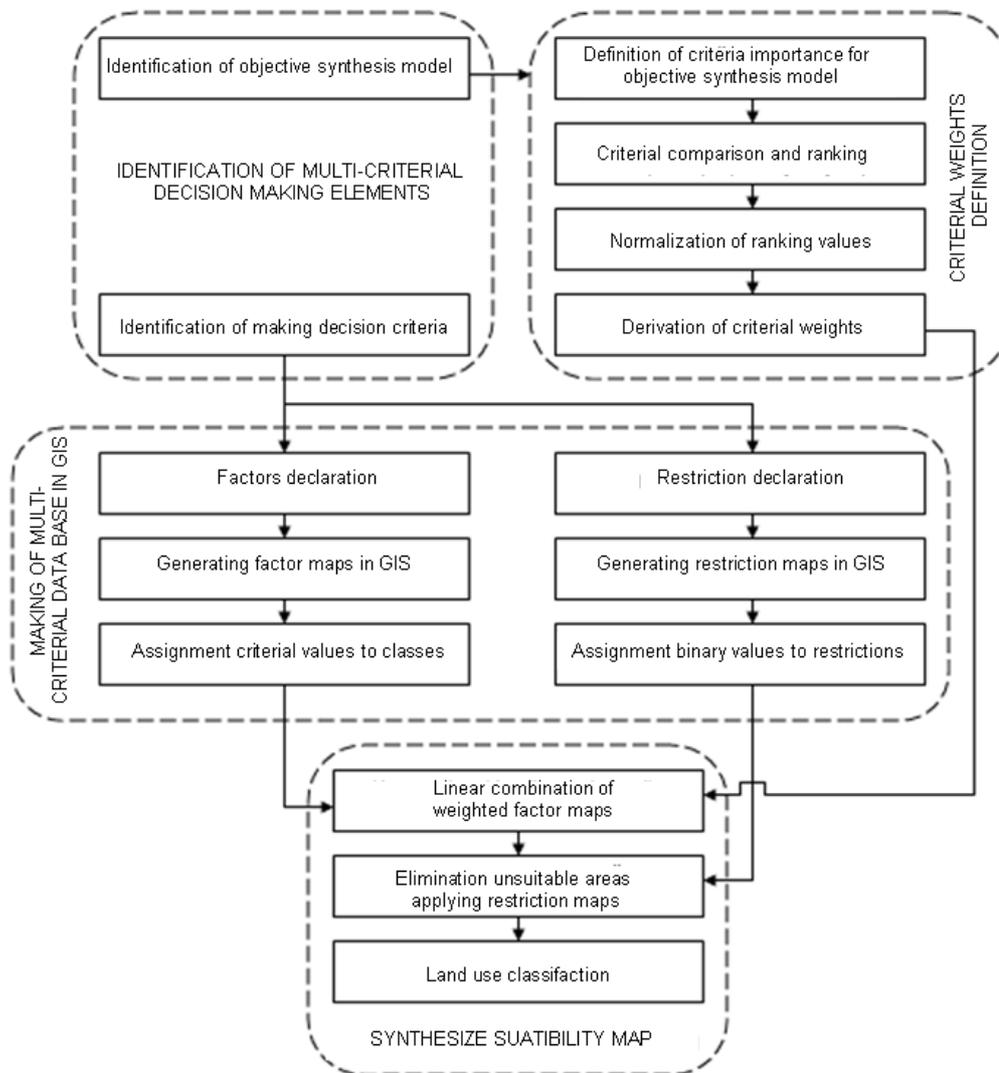
Fig. 1: Key stages in the procedure of land use classification for construction of high-rise buildings
