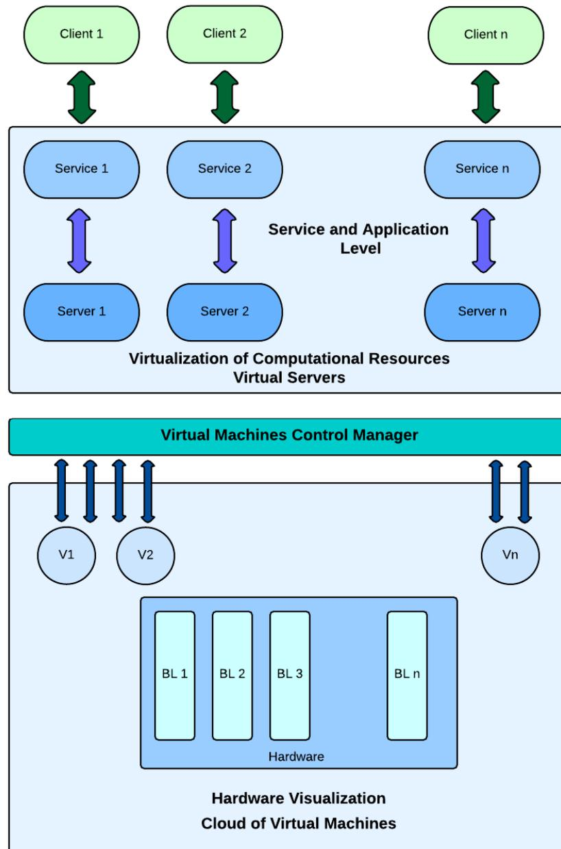
Fig. 1: Basic representation of virtualization system
