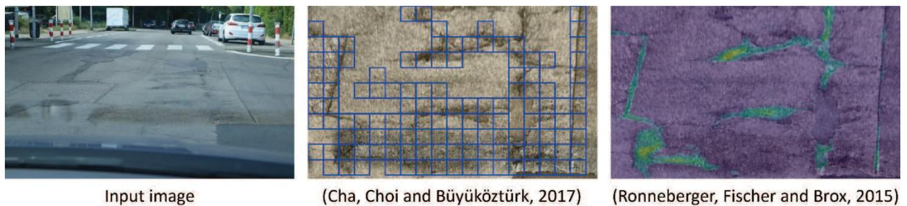
Fig. 5: Detection of cracks in the street surface. The left column shows the original input image from which the ROI is cropped using the described approach and then fed into two crack detection methods (second and third column). From these outputs, numerical features for the state of repair prediction can be derived. (Own source)
