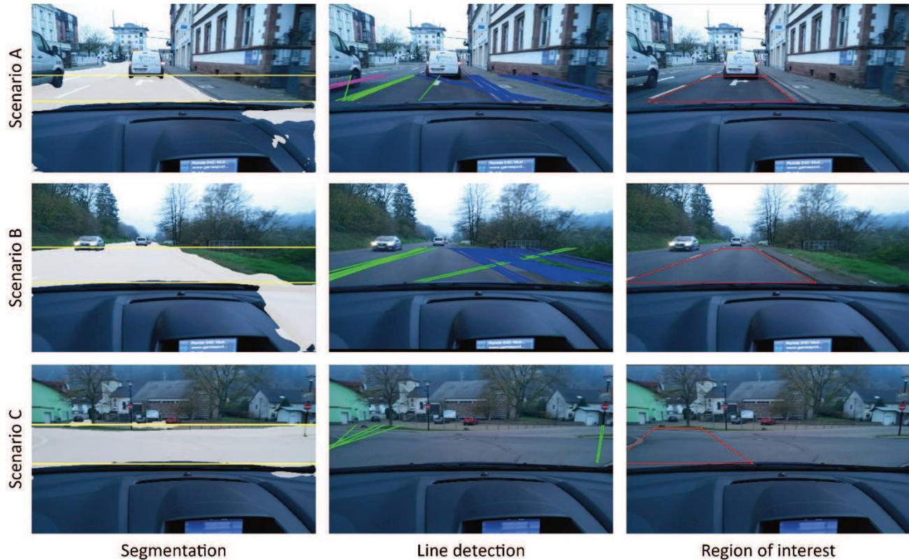
Fig. 4: Automated ROI detection. We combine information from line detection using the Hough transform (left) and a semantic scene segmentation approach based on Deep Learning that is able to detect the parts of the image pertaining to the street or road (middle) to automatically determine a quadrilateral region of interest for each image. (Own source)
