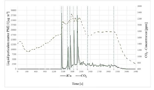
Fig. 11: Experiments in a closed room with e-cigarette: comparison of CO2 and liquid particle readings directly at the source
