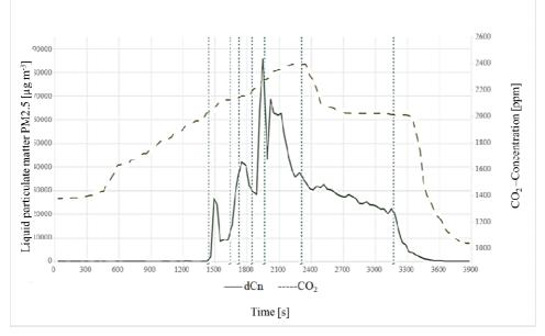
Fig. 12: Experiments in a closed room with e-cigarette: comparison of CO<sub>2</sub> and liquid particle readings approx. 2 m from the source
