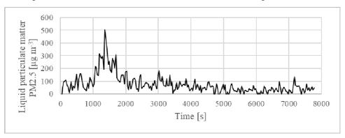
Fig. 9: Liquid particle measurement course in the entrance area during the lunch break
