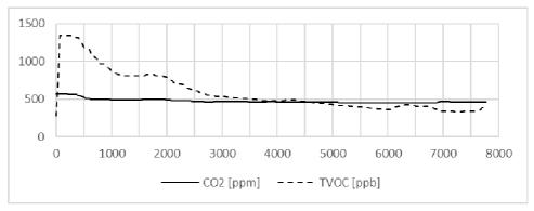
Fig. 8: CO<sub>2</sub> and TVOC measurement curves in the entrance area during the lunch break
